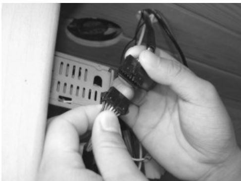
FIG-20 Link the control panel connectors
